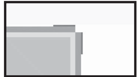
5 - Place masking tape on the ends of the slabs.
